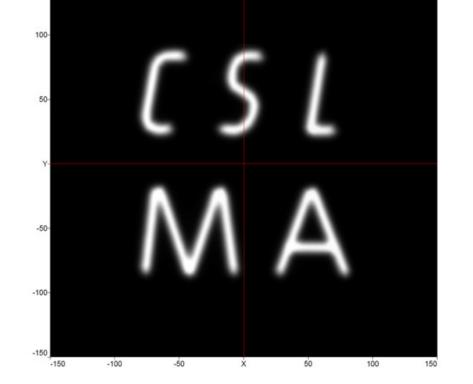
Fig. 4: Beam scan, delivered with a C-DDS prototype at MedAustron
